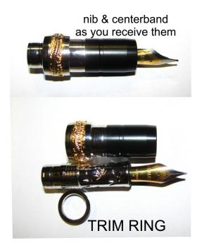
CERTAIN TO WATCH THE TRIM RING!! Do NOT lose it, we do NOT have extra parts for this pen!! Again, remember the nib "grain" should line up with the grain of the cap, at the centerband. Press the nib coupler in the end of the body tube.
