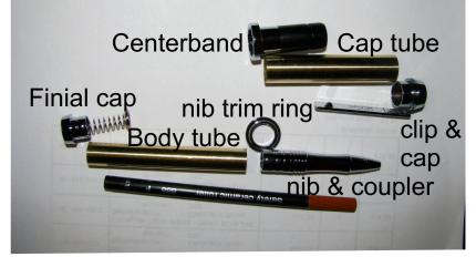
Before beginning assembly, make certain there is no glue remaining in the ends of your tubes. The first half inch of each end MUST be CLEAN. Use a small penknife or a round file to clean it out thoroughly!!! (I know I said this before, but it IS IMPORTANT!!!!!!)
