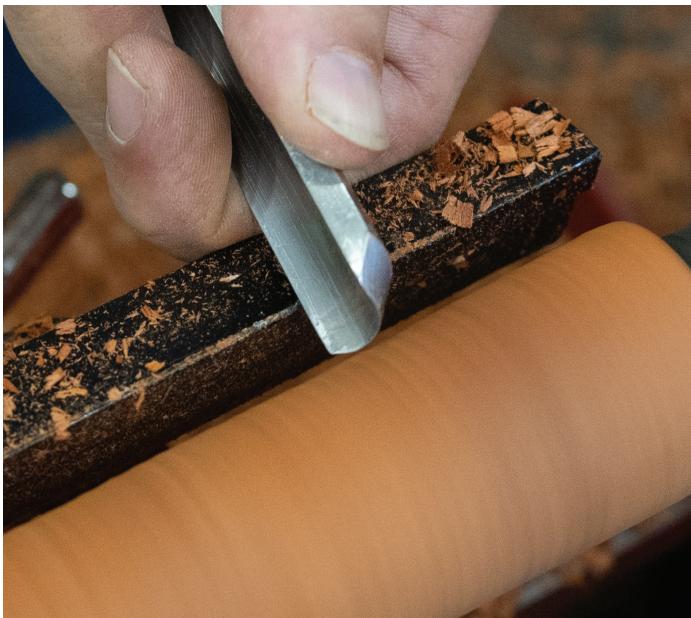
Fig 16: Start with flute facing center of intended cove
