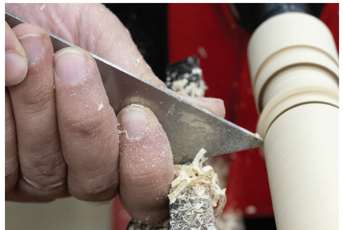
Fig 10: Scraping cut below centerline
