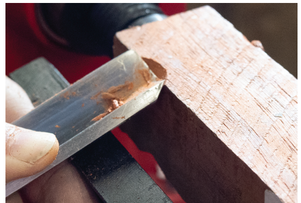
Fig 6: Bevel remains in contact with cut material
