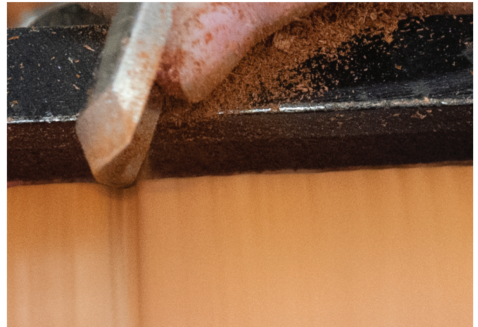
Fig 13: Twist tool so flute rolls towards the cut
