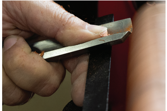
Fig 1: Holding the Chisel
