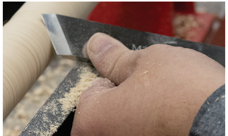
Fig 3: Planing Cut –front view. Note toe is above surface
