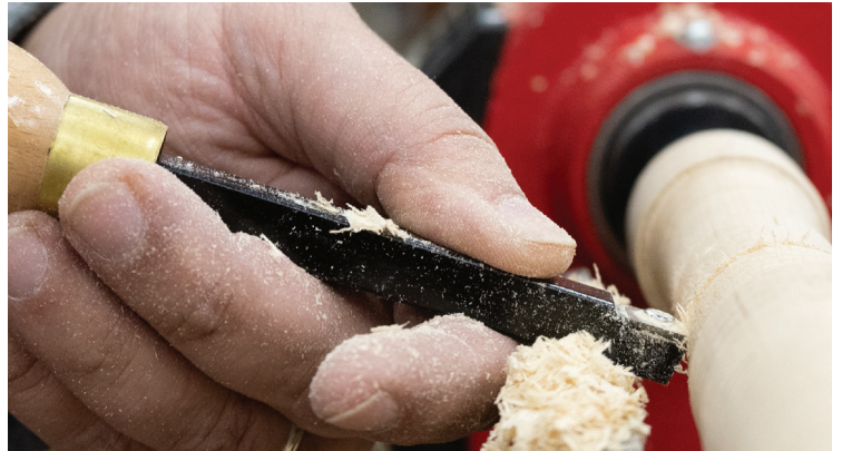
Fig 20: Holding #LCWIZ Square Cutter below center to create negative rake angle
