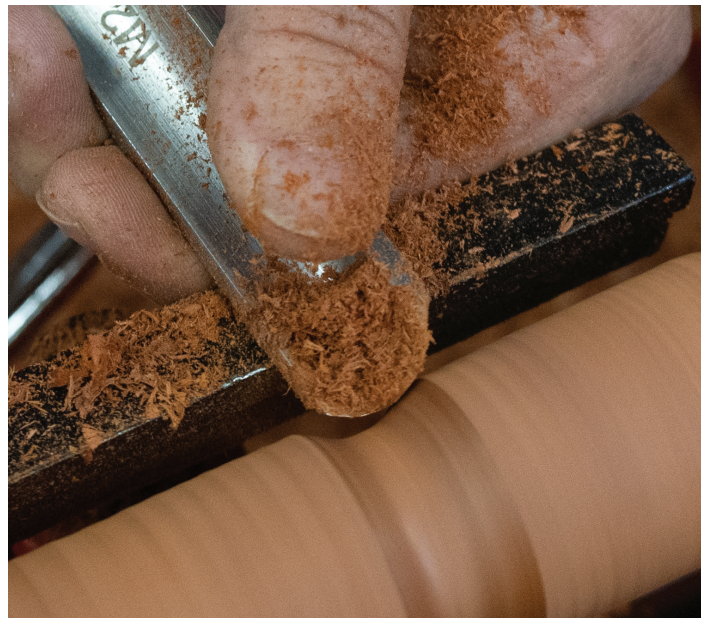
Fig 19: Both cuts meet in the middle with flute facing up
