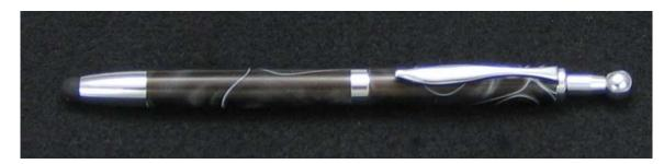
Needed: Mandrel-A Bushing Set-56A Drill-Letter "O" Blank Size- 5/8" x 5/8"
