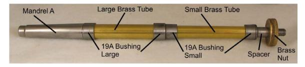
1. Assemble the blanks on the mandrel with the right bushings in the right place. The right bushing can be found by comparing the diameter of the bushing to the piece of hardware that will be placed in that place. For instance, the bushing that is the same size as the clip will fit on the end of the blank that will eventually become the top of the cap.
