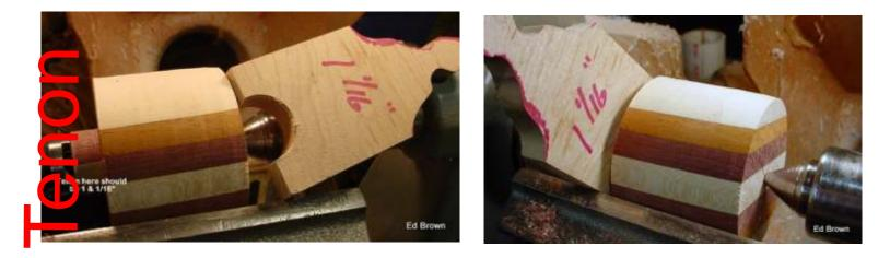
Turn top to round, making certain to turn a tenon that will fit inside your hole (this mechanism requires a 1&1/16" hole). I have made this jig to assist in getting a tenon that will fit accurately.
