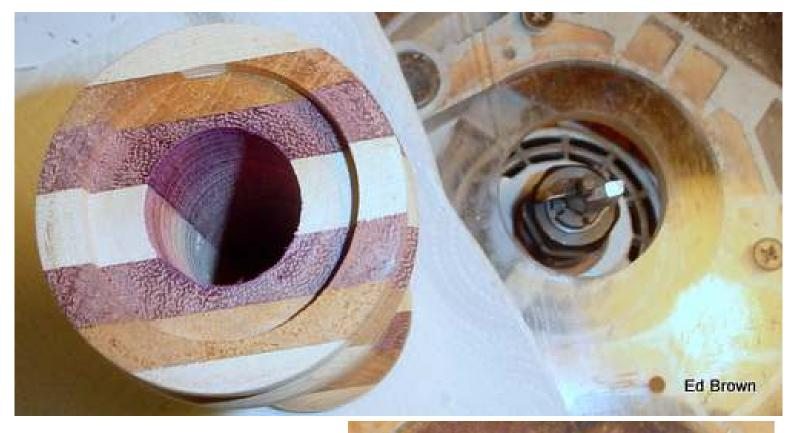
To make the indent for the "hardware" in the bottom, I use a router with a 1/4" dado bit, mounted in my router table. The table has a clear acrylic top so the picture is misleading. I use an old "paddle-type" bit The newer dado bits are too big to fit in the hole and cut the dado safely.
