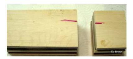
This will be an 8" mill, so I cut the blank at 6.5" and the top about 2.5". Mark the pieces so you don't forget where the pattern will match up.
