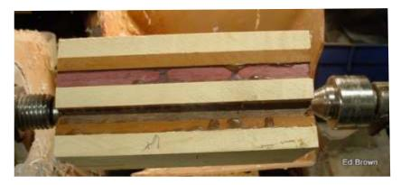
Now, mount the body between centers, making certain to hit the center of the "X" with the point of the drive center and live center in the tailstock.
