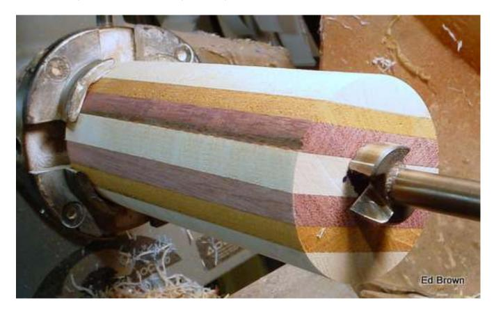
Mount the body in a scroll chuck, with the #2 jaws. Insert a 1&1/16" forstner bit into the Jacobs chuck and run the lathe about 500 RPM. Slowly push the drill bit into the body, retracting frequently to remove shavings. If bit gets very hot, stop for a while. Heat is NOT good, but does happen.
