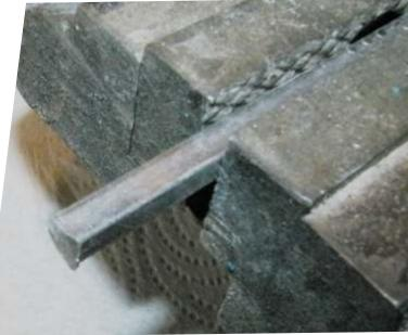
Hard to see, but the end is bent over so it will catch the male part of the grinder mechanism
