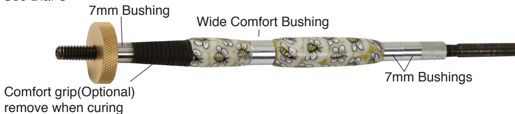
D Mold on mandrel - apply cane around tube. See Dia. C
